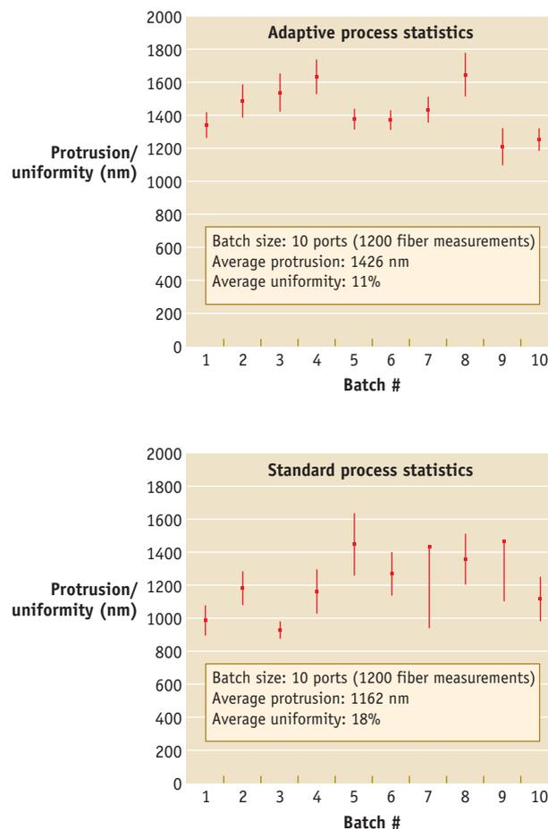
FIGURE 2. Adaptive process-control statistics (top) show more uniformity than standard time-control process statistics (bottom).
