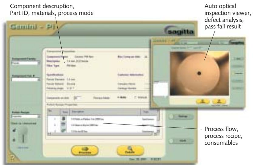
**FIGURE 3.** A user-friendly graphical user interface manages the process and system control software as well as data management for an automated polishing system. This screen image from the Sagitta Gemini system shows the operating menu and the optical inspection viewer during image processing for defect analysis.
