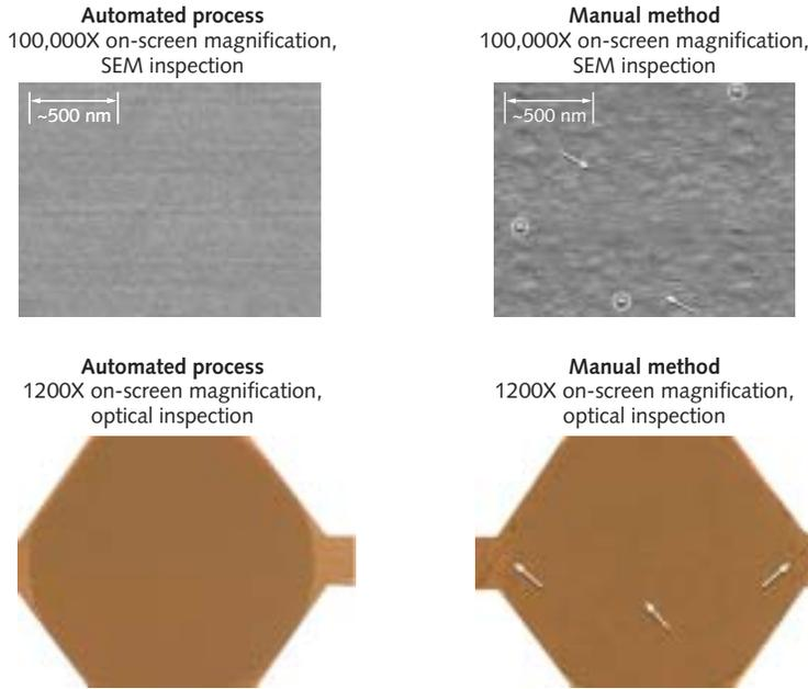
**FIGURE 2.** Automated polishing provides superior surface finish for a silica waveguide multichannel arrayed waveguide grating (top left) compared to manual polishing (top right). Similarly, for a SMF fiber in a v-groove notch the finish provided by the automated process has fewer surface defects (bottom left) than that possible with manual polishing (bottom right).
